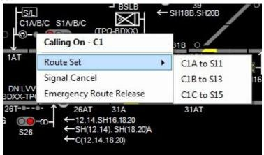
To take off calling-on signal, the train must come to a stop at the foot of the Home signal, occupying the track circuit (1AT or 2AT as the case may be) in rear of the signal. When a train occupies the track circuit, a red light strip will appear on the VDU. The particular route on which train is intended to be received shall be set by tracking the pointer in VDU on to the signal below which the calling-on signal is provided. Right click on the calling-on signal which will appear a pop-up menu.
