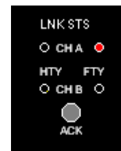
Channel - A Link Status is Faulty
