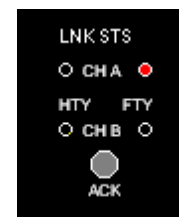
Channel – A Link Status is Faulty
