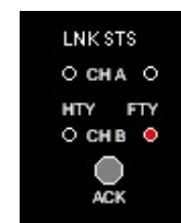
Channel - B Link Status is Faulty
