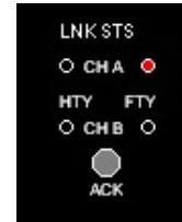
Channel - A Link Status is Faulty
