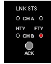
Channel – B Link Status is Faulty
