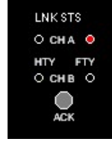
Channel – A Link Status is Faulty
