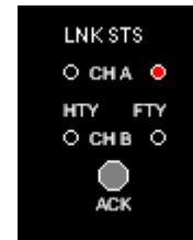
Channel - A Link Status is Faulty
