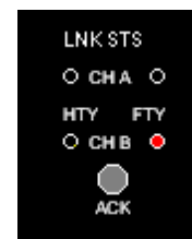
Channel - B Link Status is Faulty
