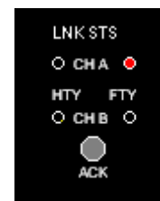
Channel - A Link Status is Faulty
