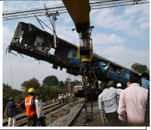
Coaches tackled at Kunderu(RV Line) on 22.1.2017 with 140ton diesel crane.
