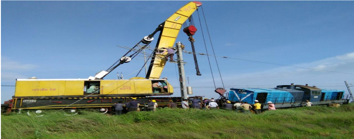
Diesel locos tackled at VPT on date 19-07-19 with 120ton diesel crane.
