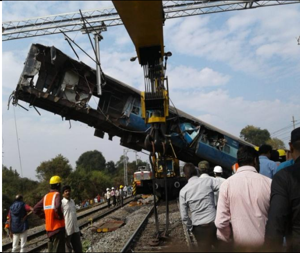
Coaches tackled at Kunderu(RV Line) on 22.1.2017 with 140ton diesel crane.
