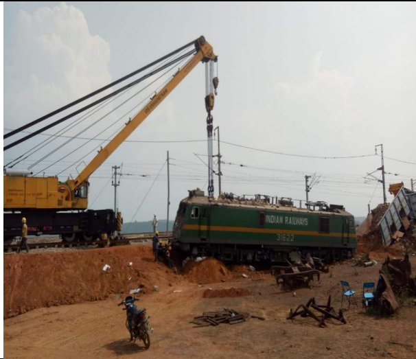
Coaches tackled at Kunderu(RV Line) on 22.1.2017 with 140ton diesel crane.
