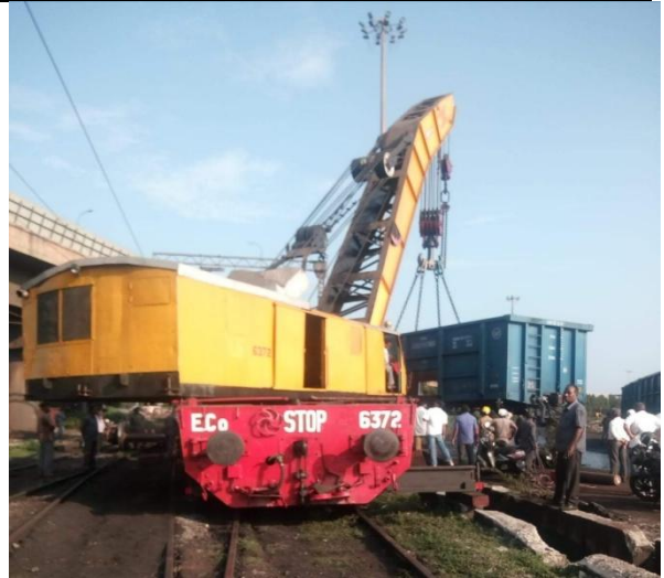
Diesel locos tackled at VPT on date 19-07-19 with 120ton diesel crane.
