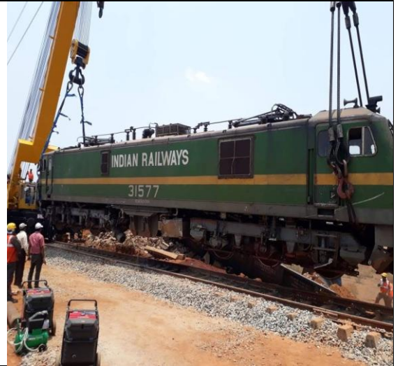
Coaches tackled at Kunderu(RV Line) on 22.1.2017 with 140ton diesel crane.
