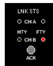
Channel - B Link Status is Faulty
