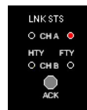
Channel - A Link Status is Faulty
