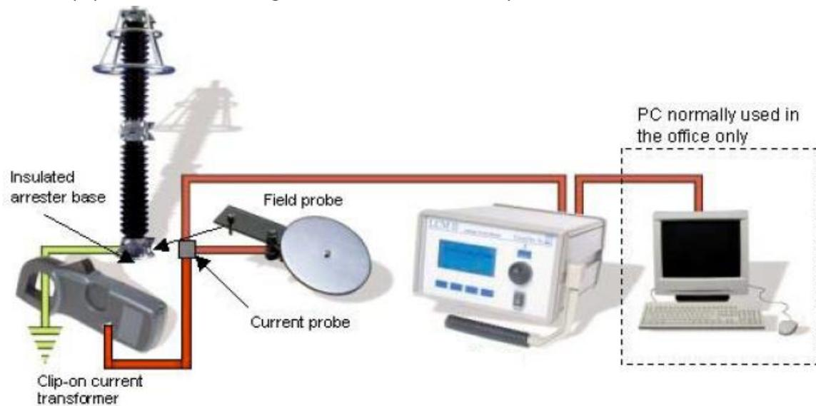
6.2.2 Assessment of resistive component of leakage current is a very sensitive measurement due to its small value (few micro amperes) and its dependence on Voltage and temperature. Every reading recorded is also accompanied by the Voltage and temperature at the time of reading.
