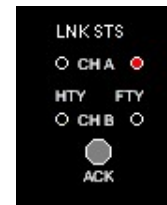
Channel - A Link Status is Faulty
