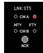
Channel - A Link Status is Faulty
