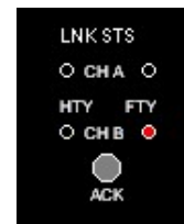
Channel - B Link Status is Faulty
