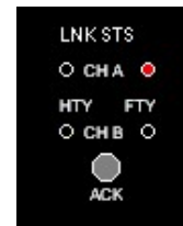
Channel - A Link Status is Faulty
