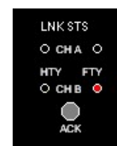
Channel - B Link Status is Faulty
