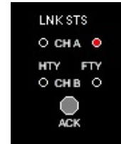
Channel - A Link Status is Faulty
