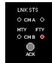
Channel - B Link Status is Faulty
