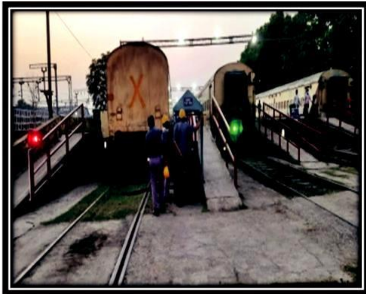
Danger lamps provided at the entrance of the Pit Lines for safety of staff during under gear examination work at night time.
