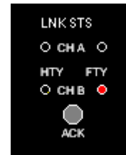
Channel - B Link Status is Faulty
