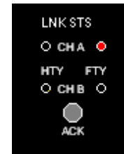
Channel - A Link Status is Faulty
