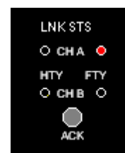
Channel – A Link Status is Faulty
